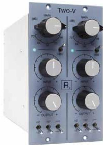
The +48 VDC phantom power switch is accompanied by a greenish-blue LED signifying that phantom power is active. The 0°/180° switch inverts the polarity, and the High Pass switch activates a 6 dB/octave high-pass filter with a 120 Hz corner frequency; Joel Cameron has evidently found the magic corner frequency and curve to create the closest thing to a perfect high pass filter. Impedance is switchable between high (1200 ohms) and low (300 ohms).
